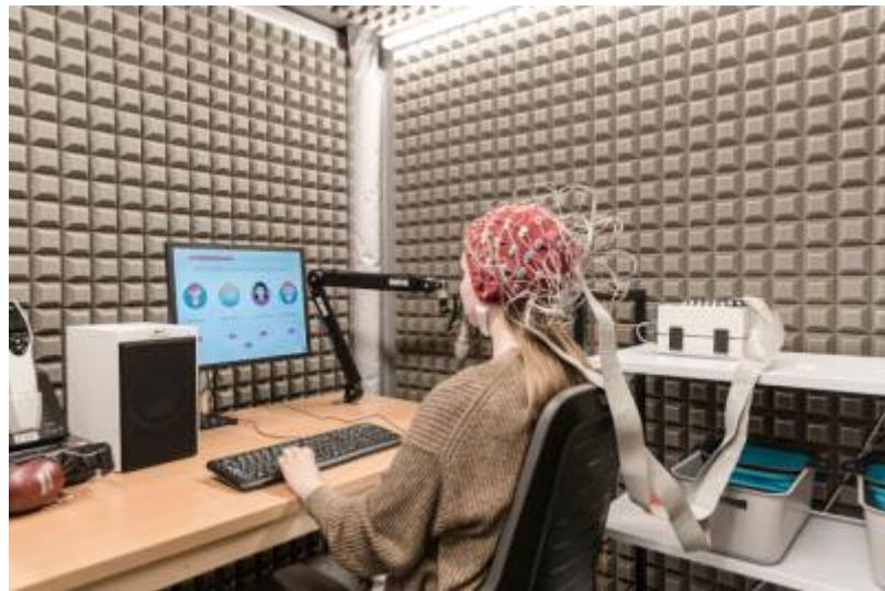
The lab is equipped with two electromagnetically shielded booths for running EEG experiments. Each booth is equipped with a *BrainProducts ActiChamp* EEG system. Each system is capable of recording 32 to 160 channels. Each booth is also equipped with a *capTack* digitisation system to record electrode position information.
