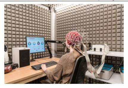
The lab is equipped with two electromagnetically shielded booths for running EEG experiments. Each booth is equipped with a *BrainProducts ActiChamp* EEG system. Each system is capable of recording 32 to 160 channels. Each booth is also equipped with a *capTack* digitisation system to record electrode position information.
