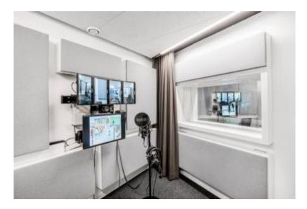
The speech lab has five acoustically treated recording booths. It is possible to record a participant in each booth simultaneously allowing for directed speech experiments with up to 5 participants. Each booth is equipped with a Røde 1000 large diaphrame condensor microphone and DT 770 head phones. Alternativly there are also DT250 headsets.
